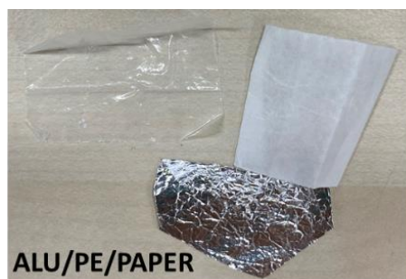
Figure 19 Image of ALU/PE/PAPER film delaminated using DES 1 – TWI.
