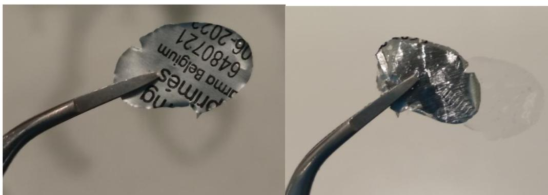
To determine the quantitative composition of the blister, a fresh sample (137.88 mg) was immersed in HCl to dissolve the aluminum and recover the other plastic layers. A thick layer of PVC (120.19 mg) was obtained, as well as the metacrylate layer (16.73 mg). The remaining mass (0.96 mg) was attributed to the thin printed metacrylate layer.
